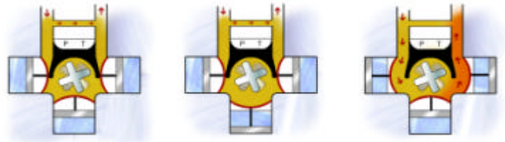
Fig. 3 Measuring principle of the CARBO 2100
